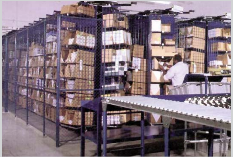
Five horizontal carousels from White help distribute almost 4000 different items. Pick rate increased from 500 times per picker/week to 2500.
