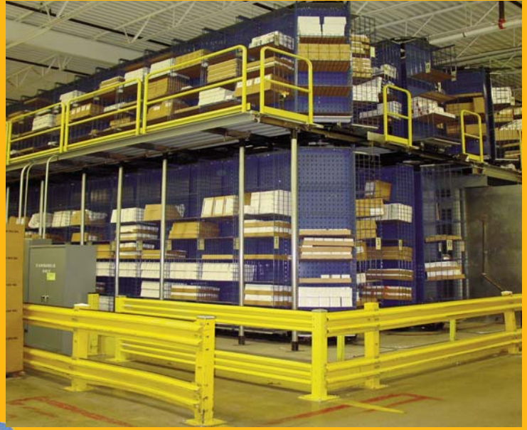
The system has 12 carousels that are configured into four picking pods.
