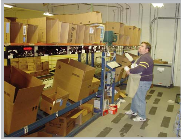
The picker is able to fill various orders at the same time. The computer software directs him which box to place the items in.
