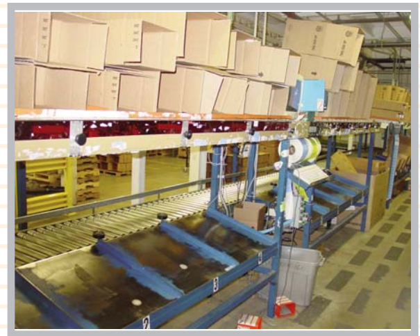
The system is designed to handle batches of eight orders picked concurrently.
