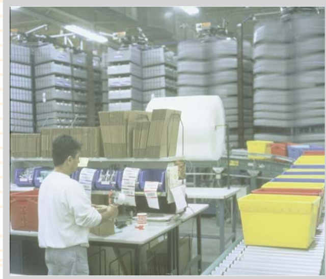
When batch picks are completed, totes move to a waiting conveyor which delivers them to the packing station.
